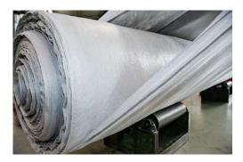
Photo 2: TenCate Geosynthetics Austria manufactures the high-strength PP nonwoven fabric shown here. The edge trimmings and production waste are processed in an ISEC evo recycling plant to produce recyclate material.
