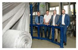
Photo 1: Even when you need to process production remnants on 5-metre-wide rolls, it's no problem for the PURE LOOP machine ISEC evo 302 E. The synthetic non-woven material is drawn in, shredded and processed into recyclate, before it can then be fed back into production.
